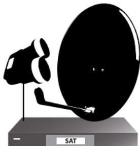
Connect the output of the Monoblock Single LNB to the input of the satellite receiver.
